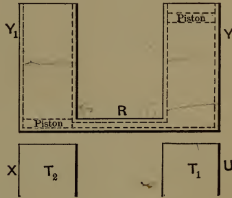
Fig. 23. — Machinery of Constant-Volume Regenerative Cycle.
